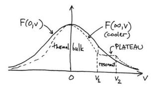
FIGURE 31. Initial stable equilibrium distribution and the final outcome of the QL evolution of a system with Landau-damped electric perturbations.
