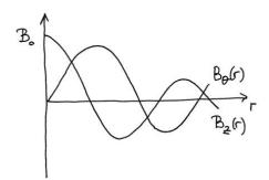
FIGURE 50. Relaxed cylindrical pinch.
