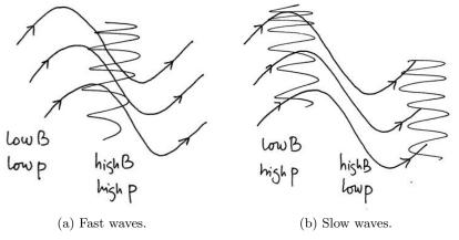
FIGURE 46. General oblique magnetosonic waves.
