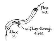
FIGURE 37. Flux tube.
